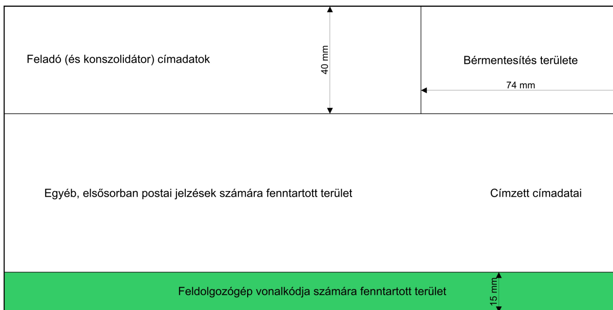
FIGURE 21: SPACE FOR THE PROCESSING BARCODE ON STANDARD AND MEDIUM-SIZED MAIL ITEMS
